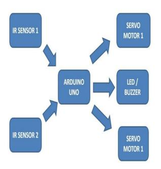
Fig:5-Block diagram of proposing model.
